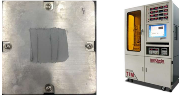
Fig.3 The fixture and thermal tester
